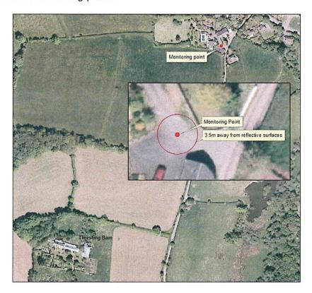
To clarify, a noise control consultant should be employed to carry out a survey to determine the typical background noise level. The background sound level, LA90, T is defined as the A-weighted sound pressure level that is exceeded by the residual sound at the assessment location for 90% of a given time interval, T, measured using time weighting F and quoted to the nearest whole number of decibels'
